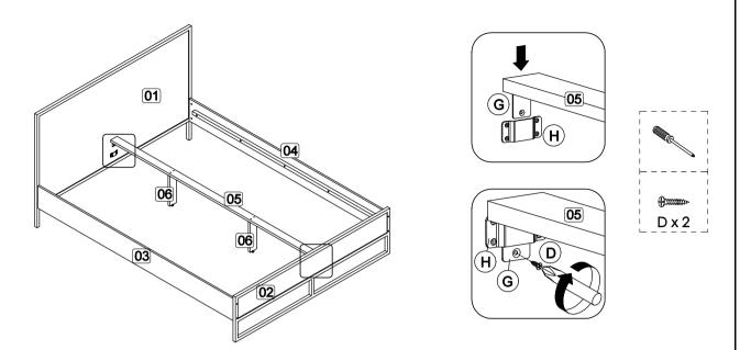
Step 5: Attach bed slat (7) to bed side rail (3), (4) and center rail (5) using hardware E with a screwdriver (not provided).
