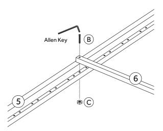
**Step 4**: Adjust both Side Supports (5) into the inner direction until the screws reach the end of the hole as shown. Tighten the screws for both Side Supports and the Mid Support.
