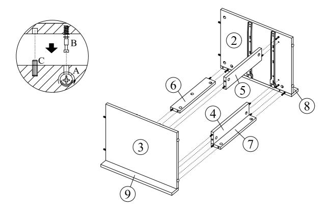
6 B 4 Insert hardware part B using a screwdriver (not provided).
