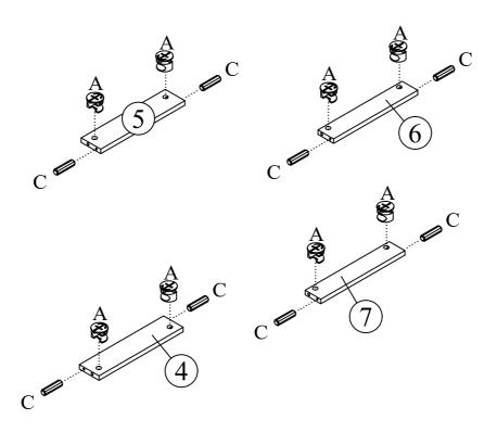
Attach the Bottom Front Panel (4) and Bottom Back Panel (5) and Top Front Post Panel (6) and Bottom Front Post Panel (7) to Left Panel (2) and Left Front Post Panel (8) and Right Panel (3) and Right Front Post Panel (9) by screwdriver (not provided).
